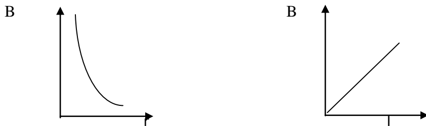
Figure 5. Variation of flux density B with radius r and current I
