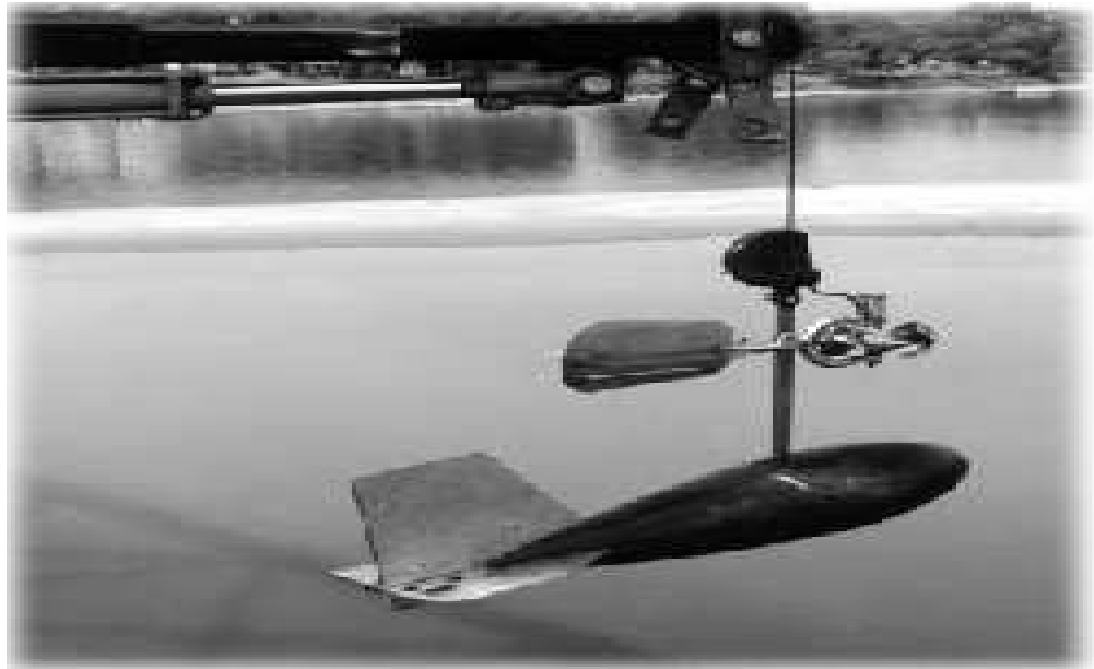
Fig. 11.3: A current meter inserted into the stream
